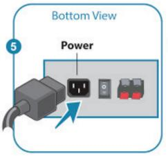
Connect power adapter to bottom **POWER** socket
