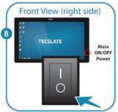
Locate main power on front right panel and switch to "ON" position
