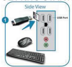
Connect wireless keyboard and mouse dongle to USB port (batteries not included)
