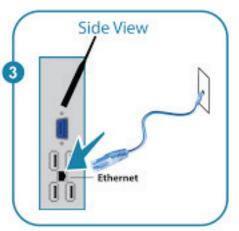
Connect Ethernet cable to Ethernet port and existing end to wall
