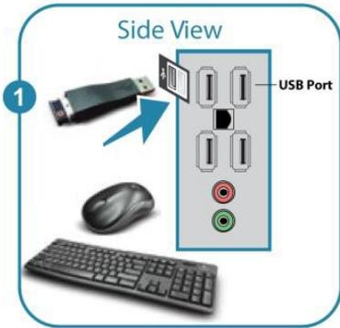
1. Connect wireless keyboard and mouse dongle to USB Port.
