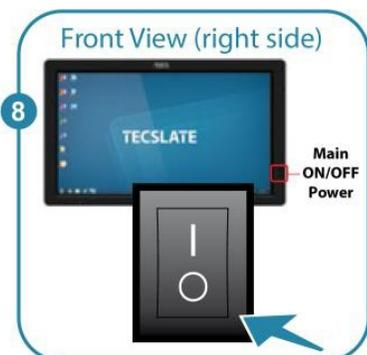
8. Locate main power on front right panel and switch to "ON" position.
