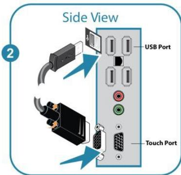
2. Connect 15 pin touch cable to TOUCH port and existing end to USB port.
